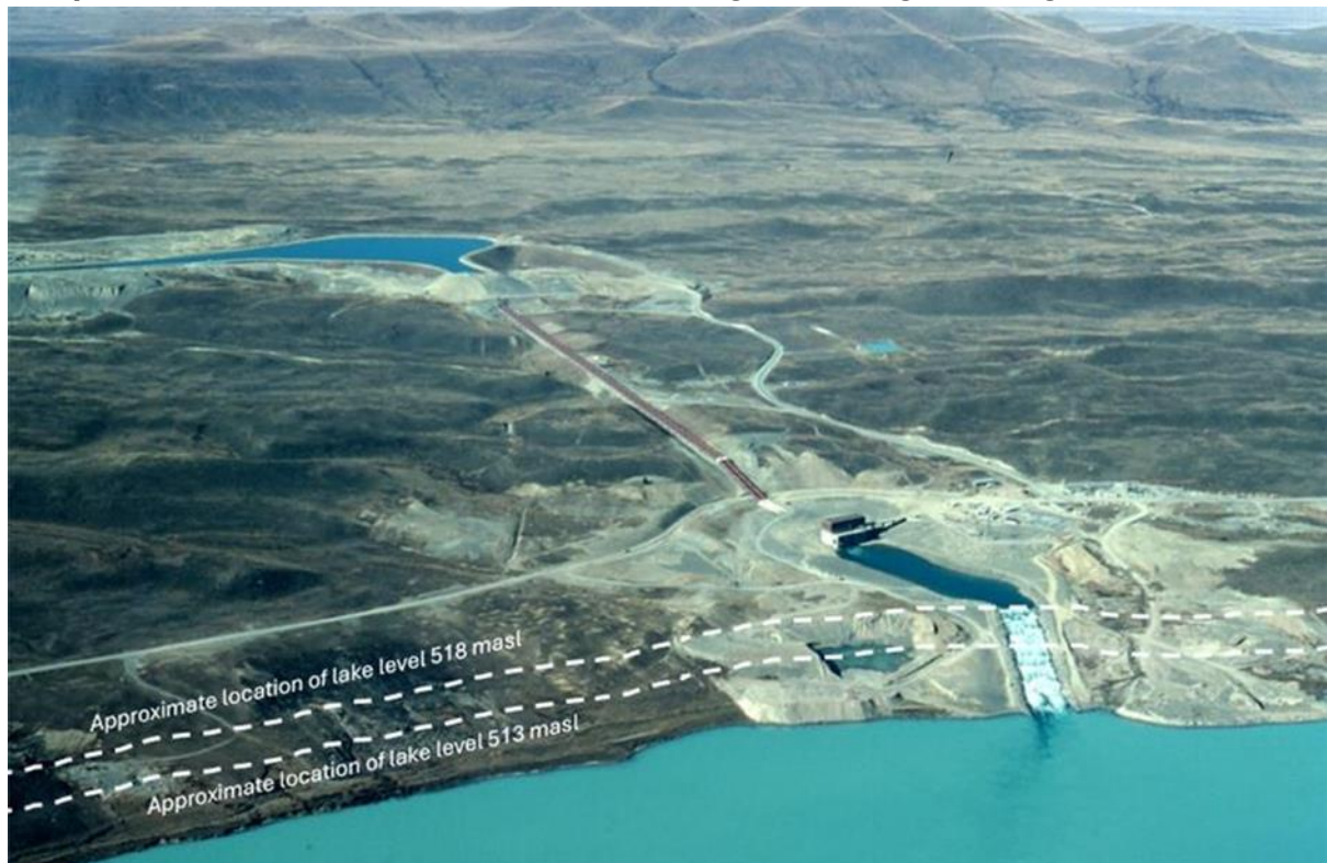
Figure 1. August 1977 – Tekapo B tailrace weir prior to Lake Pūkaki being raised following commissioning of Tekapo B Power Station. Approximate location of lake level at 513 and 518 masl indicated by dashed white line.
